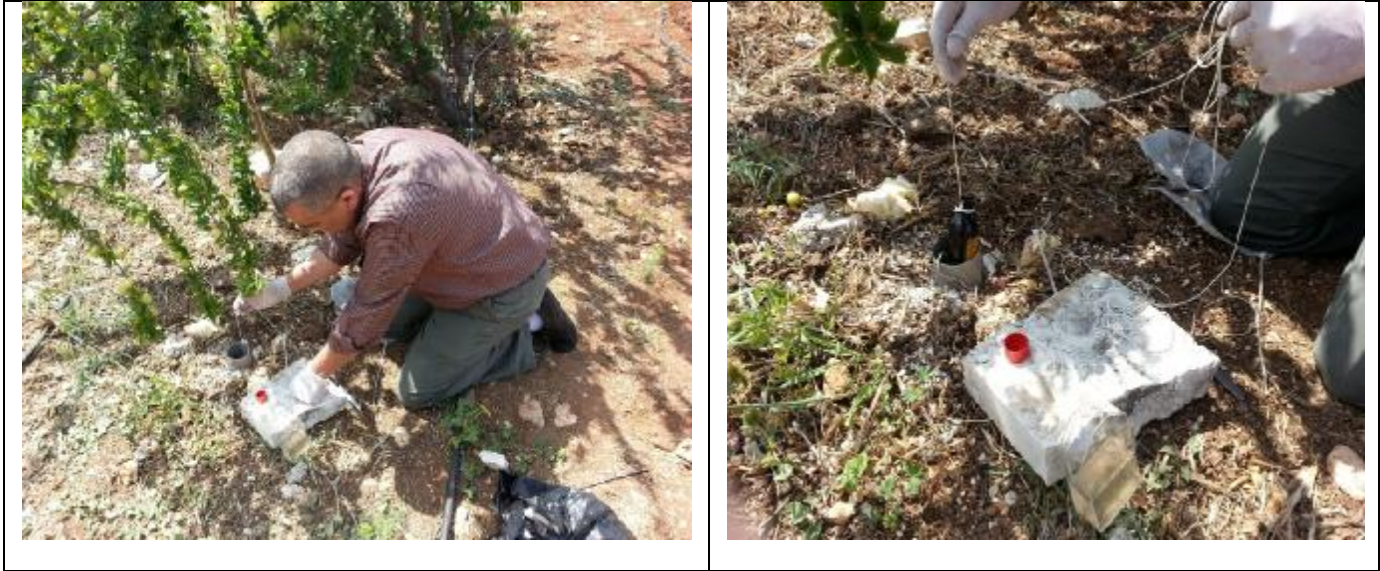
FIGURE 3-2 : SAMPLING OF INFILTRATED SEPTAGE FROM A CESSPIT IN BEIT DAJAN
